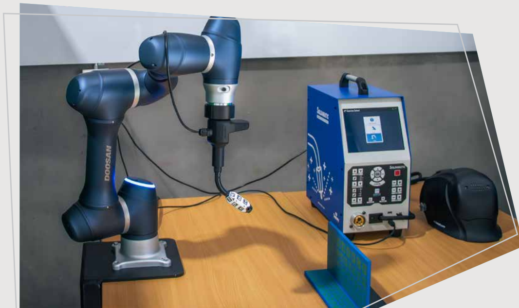
Photo caption: A cobot used with augmented reality to safely simulate welding. Photo credit: Weld Australia.
